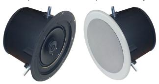
The **AMK PSA802-CFM-4-RVC** powered speakers feature a 30 watt Class D digital design amplifier, with > 75% efficiency for the main speaker. These units are available as single master speakers or sets with an unpowered companion speaker (**PSA802-CFM-4-RVC-P**) The speaker combines high performance, power handling, and a very smooth response.
